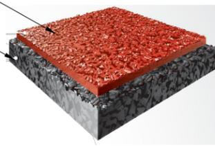
**TWO LAYER TRACK SURFACING DETAIL**
